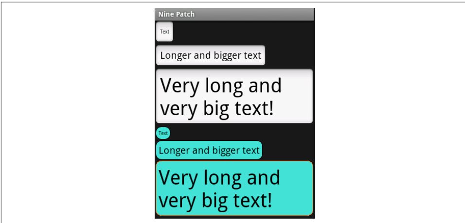
Figure 5-24. NinePatch file used as selector and background
