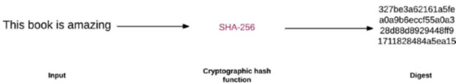
Figure 1-2. Mechanism of a cryptographic hash function. It takes an input and consistently converts it to a string of an output digest.
