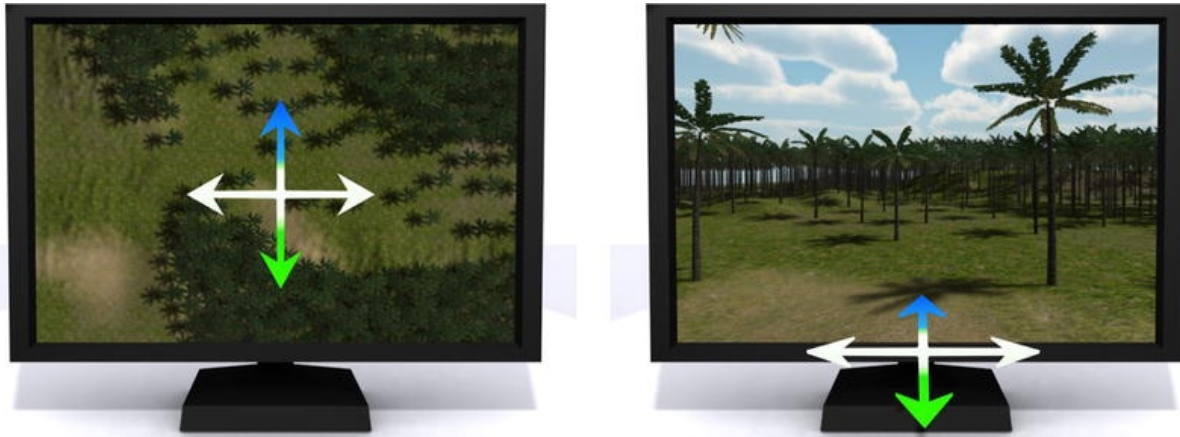
Figure 5-12. The origin of Unity navigation terminology. Left: The overhead view of a world where Vertical (on the monitor) moves you forward through the scene. Right: The directions tilted down to use in a 3D world
