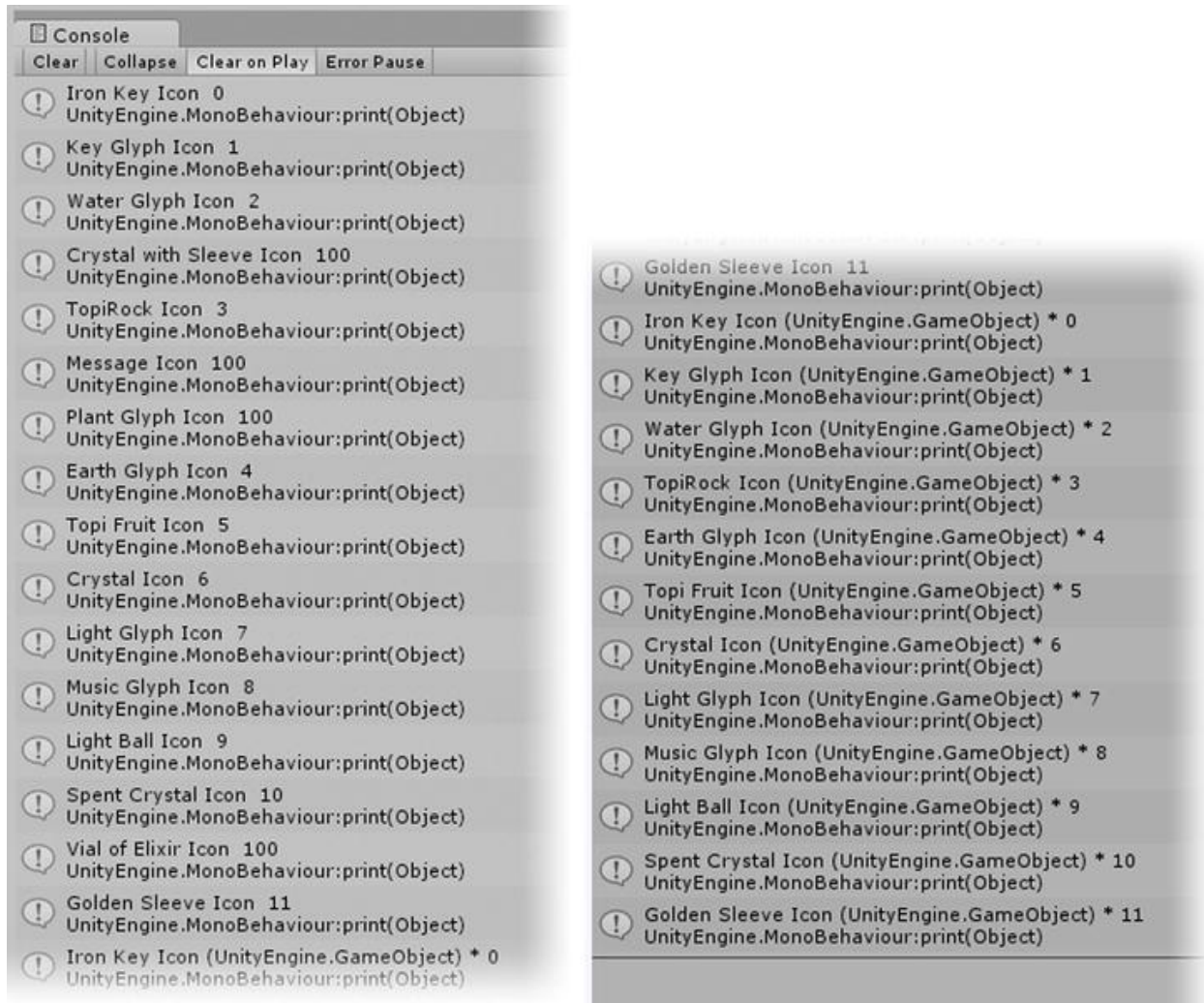
Figure 14-6. The tagged inventory objects and their newly assigned element numbers (left), and the contents of the newly generated currentInventoryObjects array (right)
