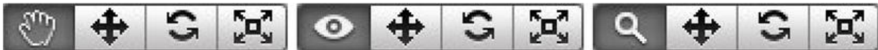
Figure 2-15. Scene navigation tools, pan, orbit, and zoom, (far left of each of the transform buttons)
