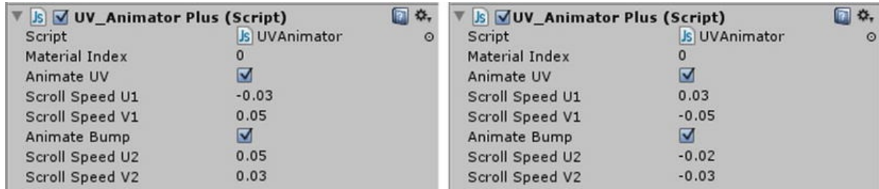
Figure 17-16. The settings for the Water Hole (left) and Water Hole Radial (right)
