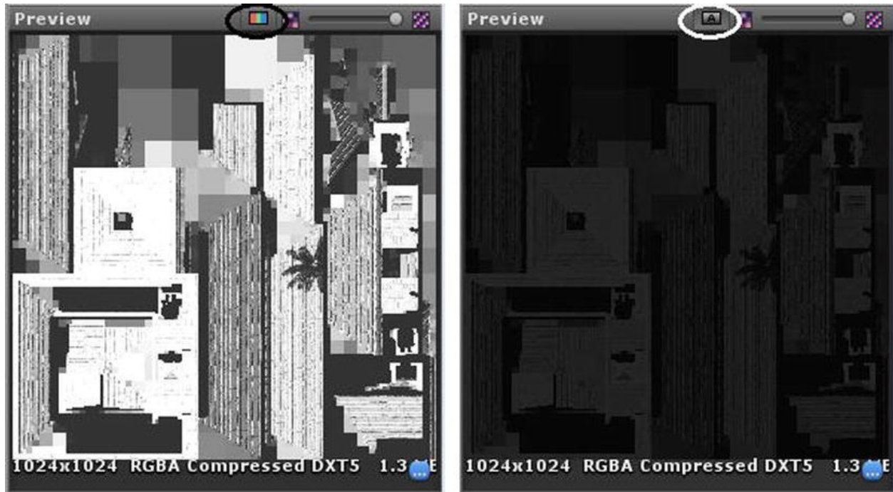
Figure 17-7. The lightmap and its alpha channel
