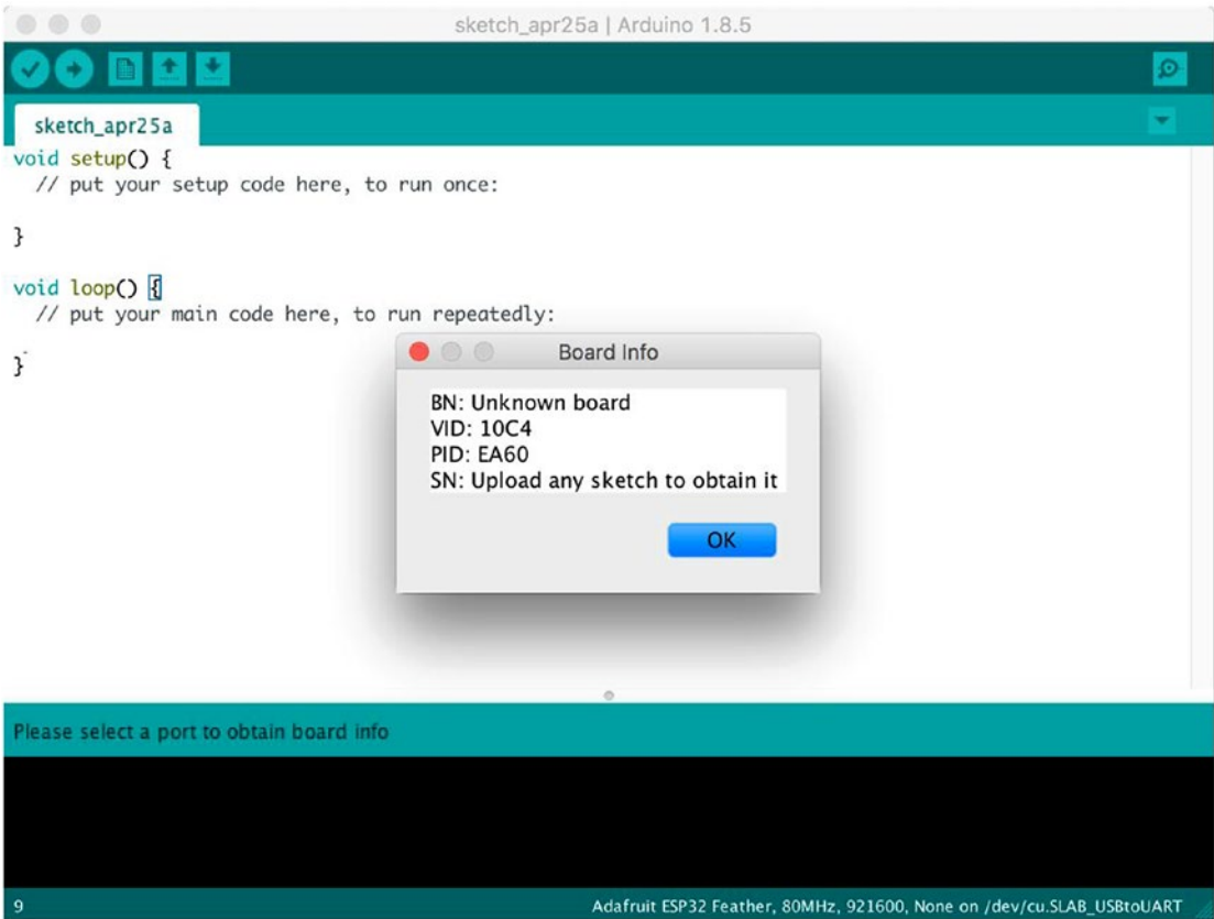
Figure 5-17. Verifying the connection to the HUZZAH32
