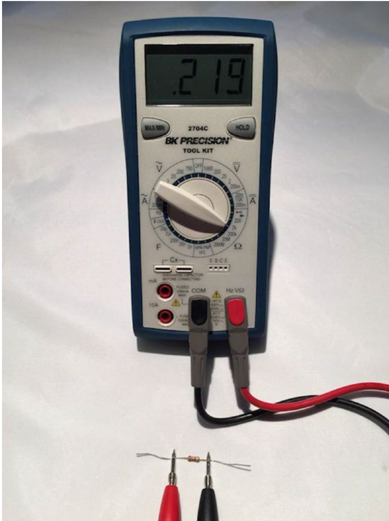
Figure 7-11. Measuring resistance of a resistor
