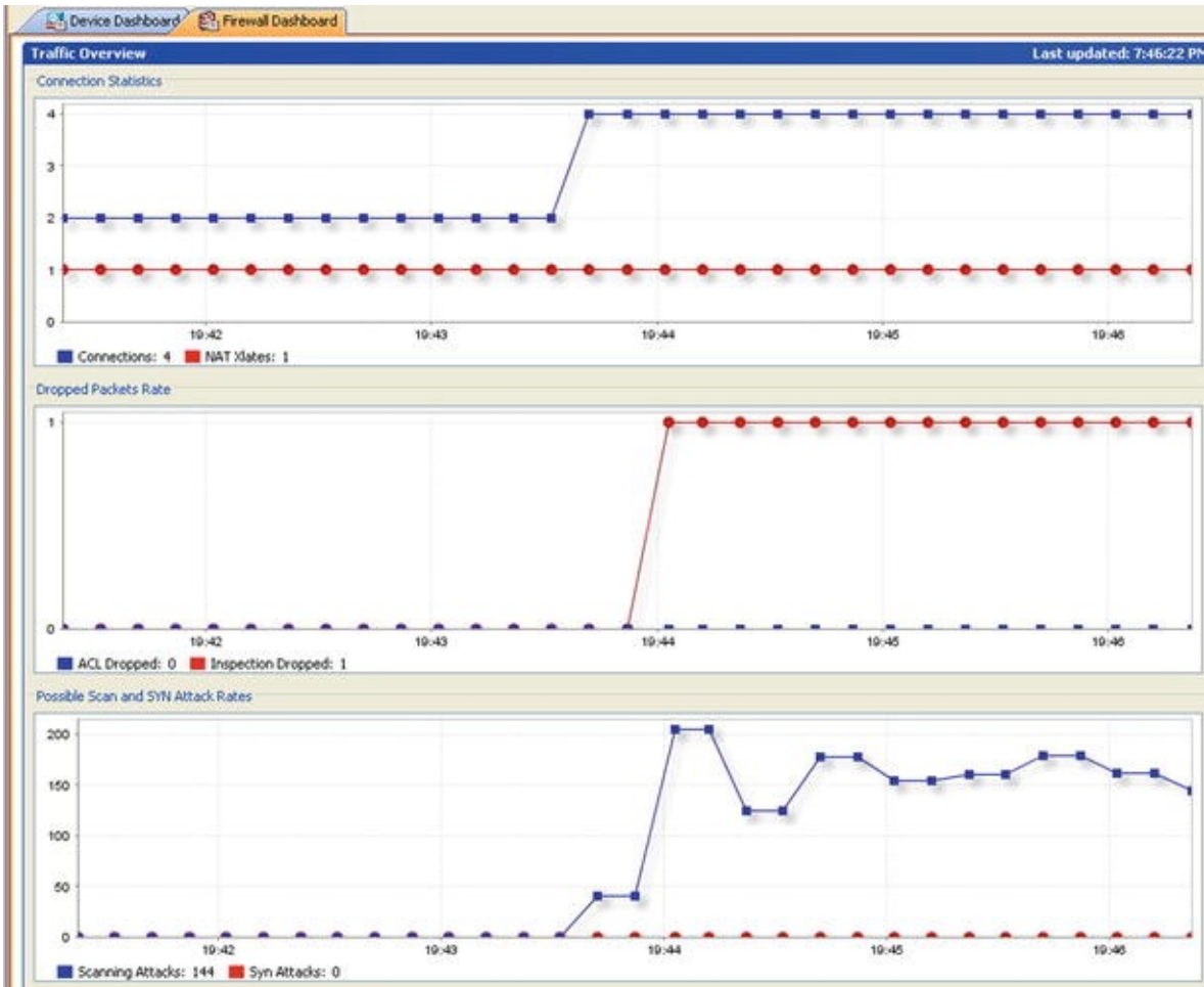
Figure 21-44. Effect of DoS with tuned connection settings and TCP normalization map is used
