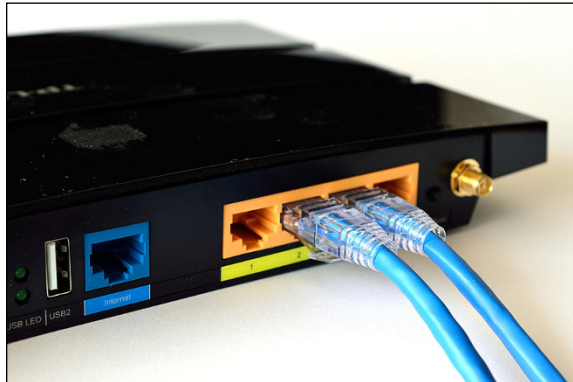
FIGURE 1-12: The back of a home router.
